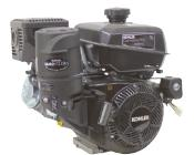
• New, KOHLER Command Pro series horizontal shaft engine. Engine features overhead valves, cast iron cylinder liner, dual ball bearings, mechanical governor, electronic ignition, fuel valve and easy to use controls. Four stage air cleaner. Automatic low oil shutdown system. EPA and California EXH/EVP SORE compliant.
