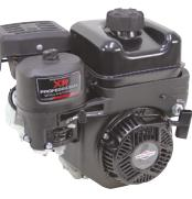
• New, BRIGGS & STRATTON XR950 Professional series engine. Features include cast iron cylinder sleeve, electronic ignition, overhead valves, ball bearing crankshaft, air cleaner, manual or remote throttle, manual choke, muffler, fuel shut off valve. EPA and California EXH/EVP SORE compliant.
