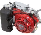
• New, HONDA GX series horizontal shaft engine. Replacement engine for generator use and other applications using a tapered shaft. Engines feature overhead valves, cast iron sleeve liner, ball bearing supported crankshaft, mechanical governor, low-oil sensor, electronic ignition, ON/OFF switch and solenoid operated Eco Throttle to control engine RPM from idle to rated speed. No muffler or fuel tank.
