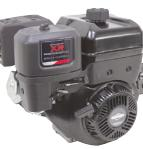
• New, BRIGGS & STRATTON XR Professional series horizontal shaft engine. Engine feature overhead valves, cast iron sleeve liner, ball bearing supported crankshaft, muffler, mechanical governor, electronic ignition, fuel valve and easy to use controls. Not for sale in California.
