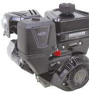
• New, BRIGGS & STRATTON Vanguard commercial series engine. Features include cast iron cylinder sleeve, float carburetor, electronic ignition, overhead valves, air cleaner, compression release, engine mounted controls, accessory mount and fuel shut off. EPA compliant and California EXH/EVP SORE compliant.
